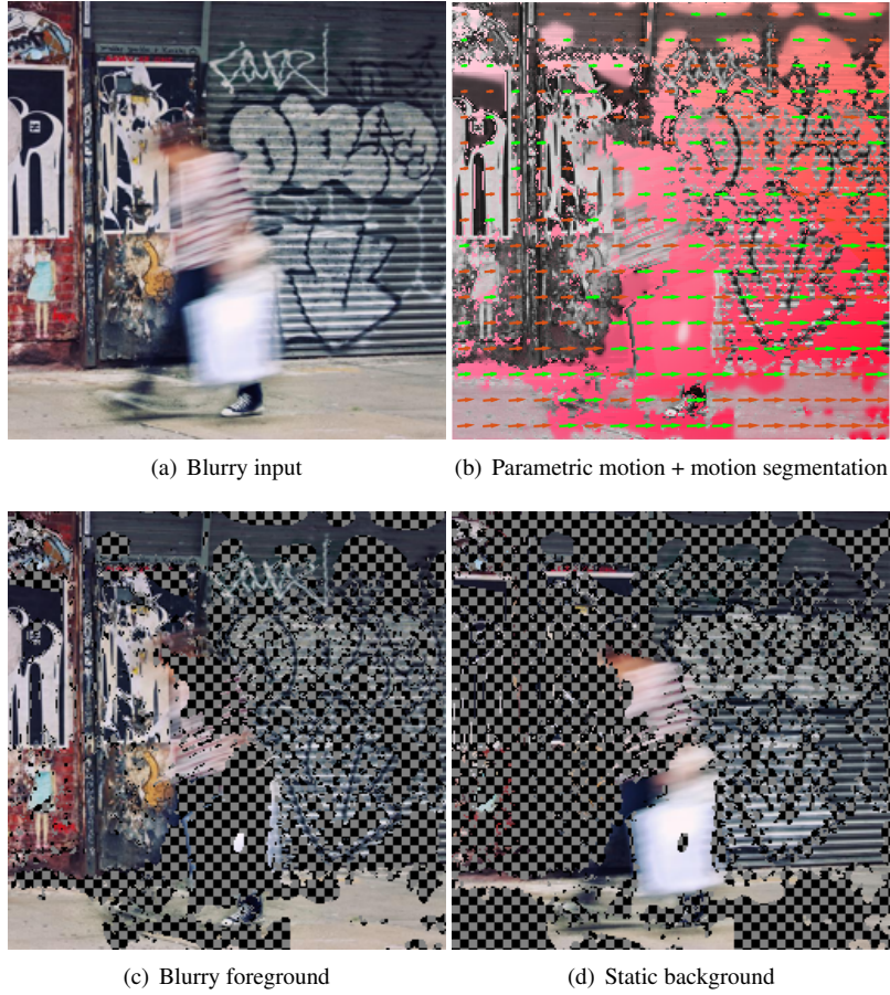
Figure 14. Motion estimation may fail if the blurry region is too small in comparison to the background.
